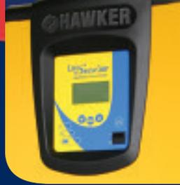
Data stored in the Battery Boss can be downloaded quickly and simply by infrared communication with a personal digital assistant device (PDA.) Using Tracker software, the PDA can hold many thousands of events, satisfying even the largest fleets. Using Profile software, the PDA can also download all charging data directly from the LifeSpeed 3000.
